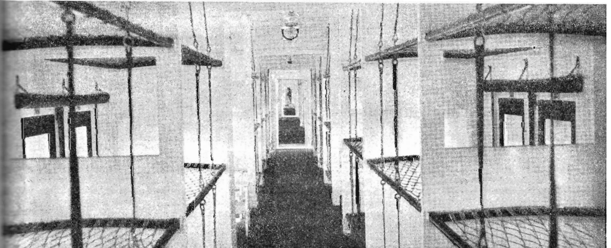
Interior of the Ambulance Train showing the tiers of bunks, the windows specially painted for service under blackout conditions and the long vista of the central corridor providing for rapid communication from one car to the other.
